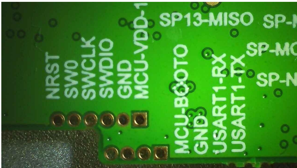
UART programming port and BOOT0 pin.
