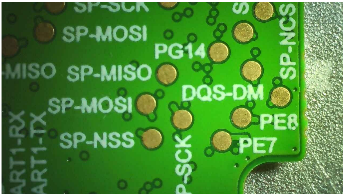
Test points and labels on the pre-production PCB.
