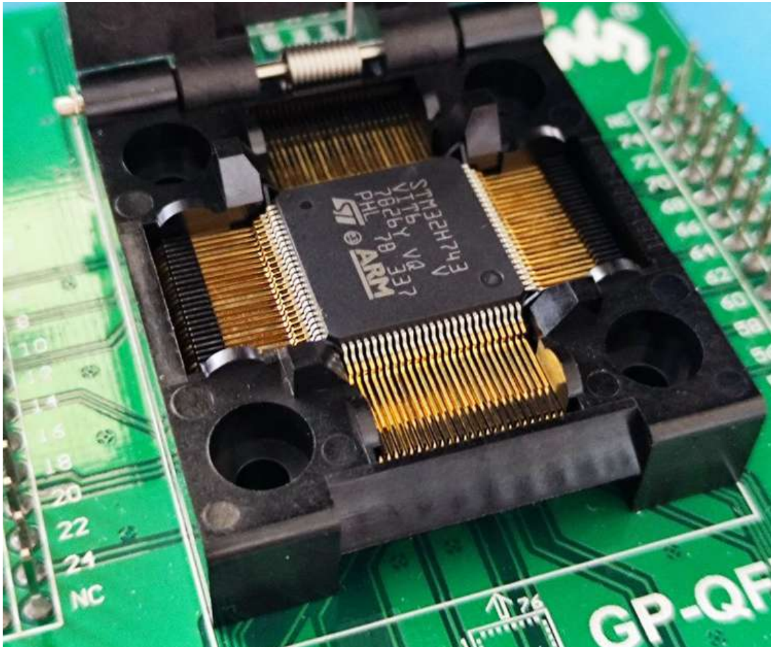
The STM32H7VIT6 in a socket for testing.
