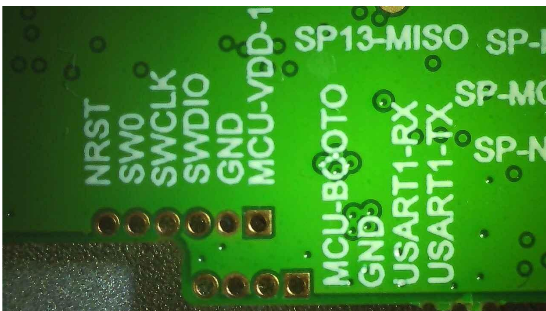
SWD header accessible at the edge of the pre-production PCB.
